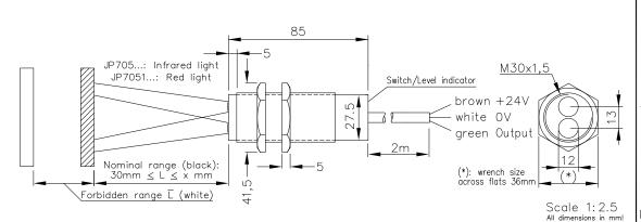
Diffuse Reflective surfaces are themselves reliably recognizable under beam incidence angles which sharply deviate from 90°.
