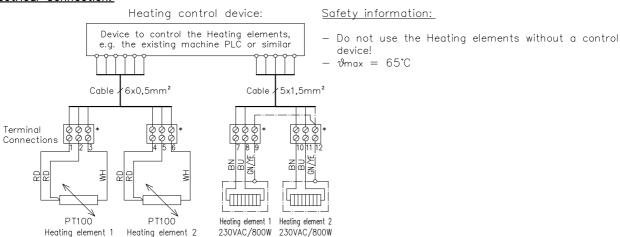
\*: You have to remove the Coupler (Kupp12GFK 0-4071) first to connect the terminal connections
